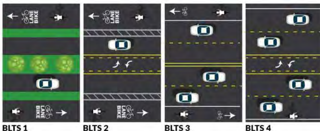
Figure 3-7: Bicycle level of traffic stress (BLTS) is illustrated by associating user types with examples of types of facilities that they feel comfortable using. The BLTS 1 scenario shows facilities that are likely to appeal to 100 percent of people who want to ride a bicycle. For BLTS 2 the facilities include buffered bike lanes which offer more separation than standard bike lines, but no physical barrier. 81% of bicycle riders would use this facility. For BLTS 3 standard bike lanes are provided and about 12 percent of riders would use this facility. Only about 1 percent of riders would use BLTS 4 facilities where no separated space is offered.
