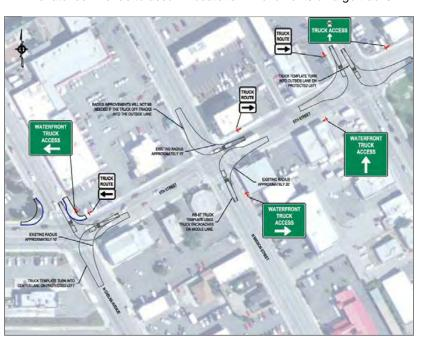
As an alternative, large trucks turning to/from on 5th Street would be allowed to continue to off-track into adjacent travel lanes.
