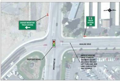
Traffic signals are recommended to make it easier for trucks to make left turns to/from 3rrd Street SE at Rock Island road and Highline Drive.
